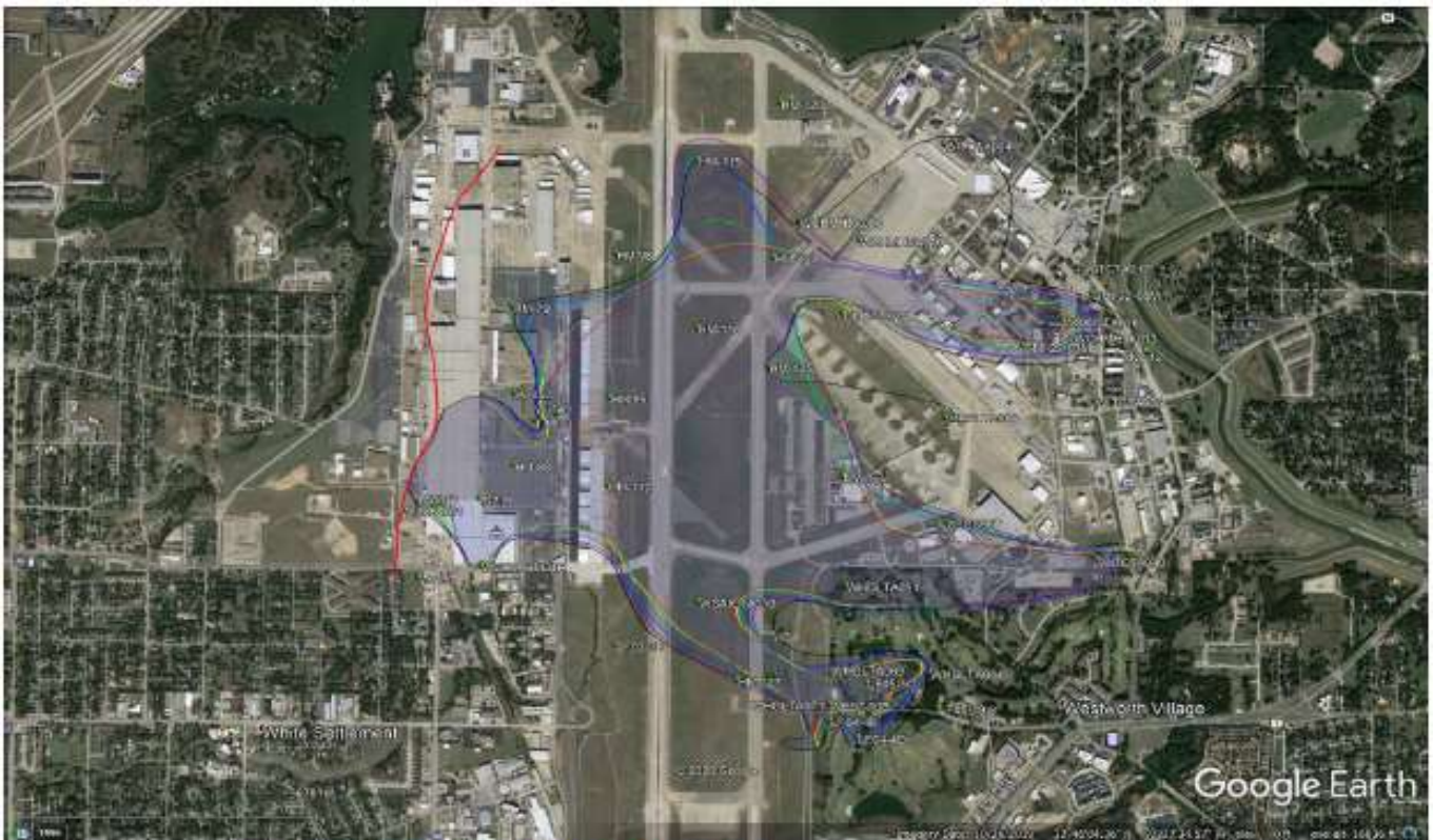
Plumes by year: 2004 2010 2012 2014 2016 2018 2020 (Red line is Terrace Alluvium groundwater divide) Plumes based on using the 2020 plume maps from the Final Biennial Groundwater Remediation Performance Monitoring Report Air Force Plant 4 (LKR, August 2020) as a starting point.
